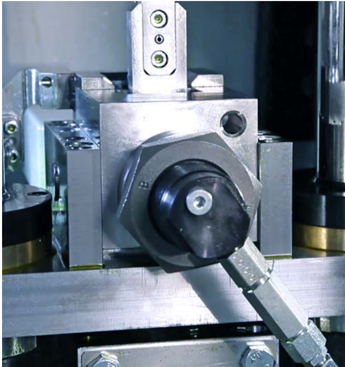
Picture: Hydraulic clamping system for the cutter bar
