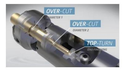
Over-Cut+ tools - have no competition when it comes to machining elongated work pieces of 1.5 mm onwards
